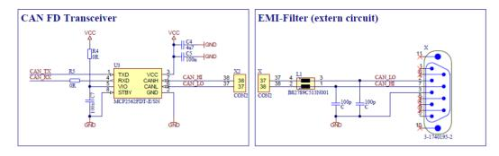
Figure 6: Design for common mode choke, recommendation
