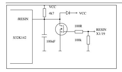
Figure 4: structure of /RESIN Line
