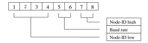
Figure 3: DIP-switch Pinout and Functions, version 3301002 only, currently not available
