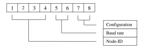
Figure 2: DIP-switch Pinout and Functions
