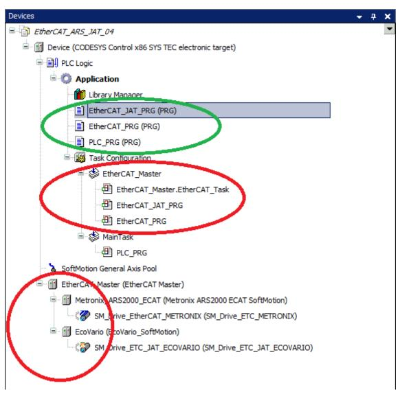
Figure 2: Device tree of the example
