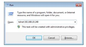
Figure 9: Calling the Telnet client in Windows
