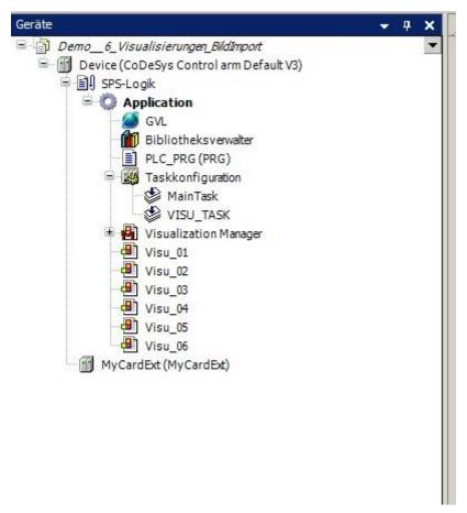
Figure 5: Device tree when using visualization in CODESYS
