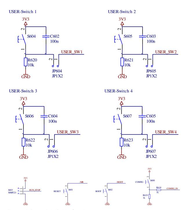
Figure 22: Reference design for User Controls
