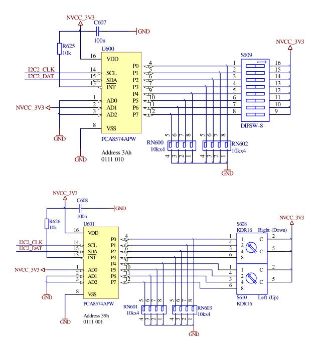
Figure 28: Reference design HEX- and DIP-Switches
