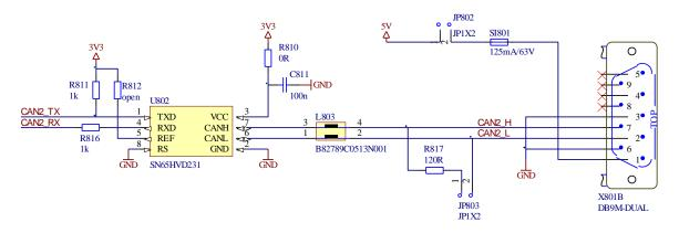
Figure 24: Reference design for interface circuits CAN
