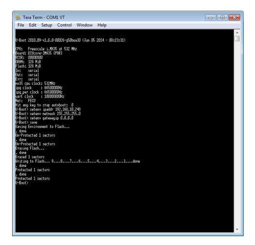
Figure 8: Ethernet configuration of the PLCcore-iMX35
