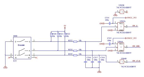
Figure 27: Reference design for Matrix Keypad and Scrollwheel
