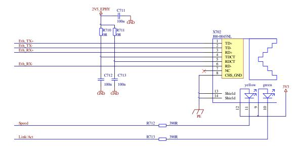
Figure 26: Reference design for interface circuit Ethernet
