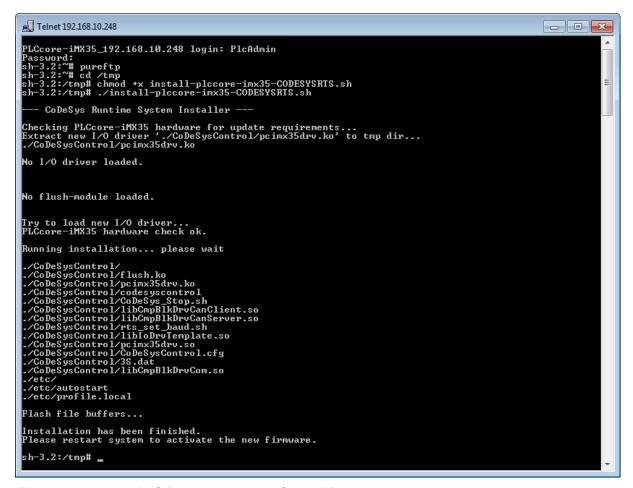
Figure 19: Installing PLC firmware on the PLCcore-iMX35
