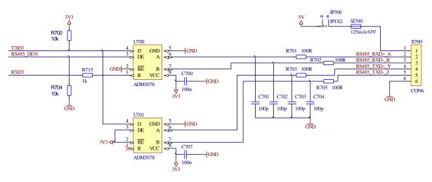
Figure 25: Reference design for interface circuits RS232/485
