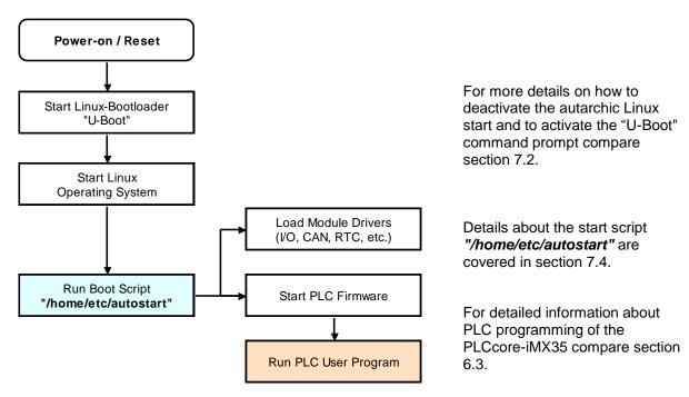
Figure 6: System start of the PLCcore-iMX35
