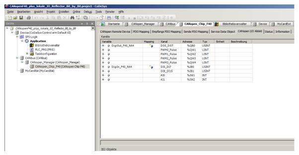
Figure 4: Variable mapping of the F407 module
