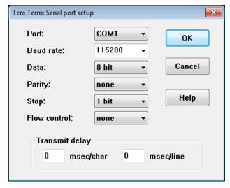
Figure 7: Terminal configuration using the example of "TeraTerm"
