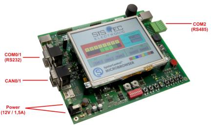
Figure 3: Positioning of most important connections on the Development Board for the PLCcore-iMX35
