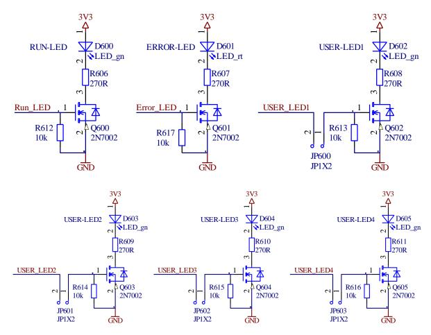
Figure 23: Reference design for LEDs
