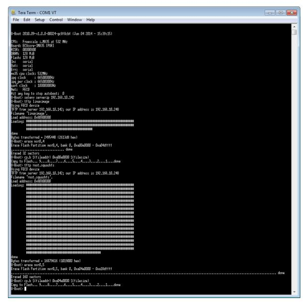
Figure 21: Downloading the Linux-Image to the PLCcore-iMX35
