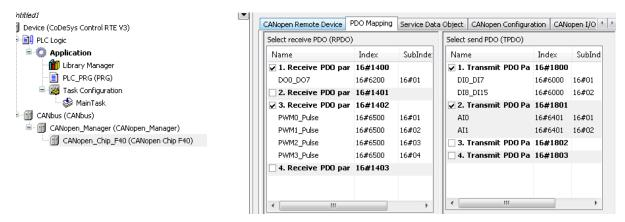
Figure 3: Default configuration of the SYSTEC F40 module
