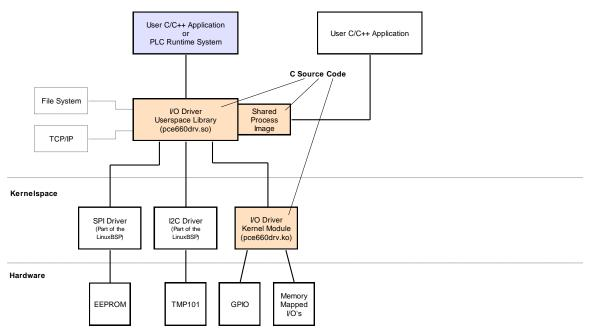
Figure 29: Overview of the Driver Development Kit for the ECUcore-E660
