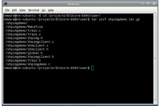
Figure 25: Unzipping the archive files shpimgdemo.tar.gz in the Linux development system
