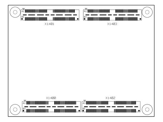
Figure 5: Pinout of the PLCcore-E660 - top view
