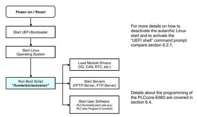
Figure 7: System start of the PLCcore-E660
