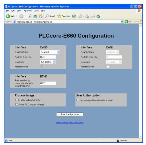
Figure 12: PLC configuration via WEB Frontend
