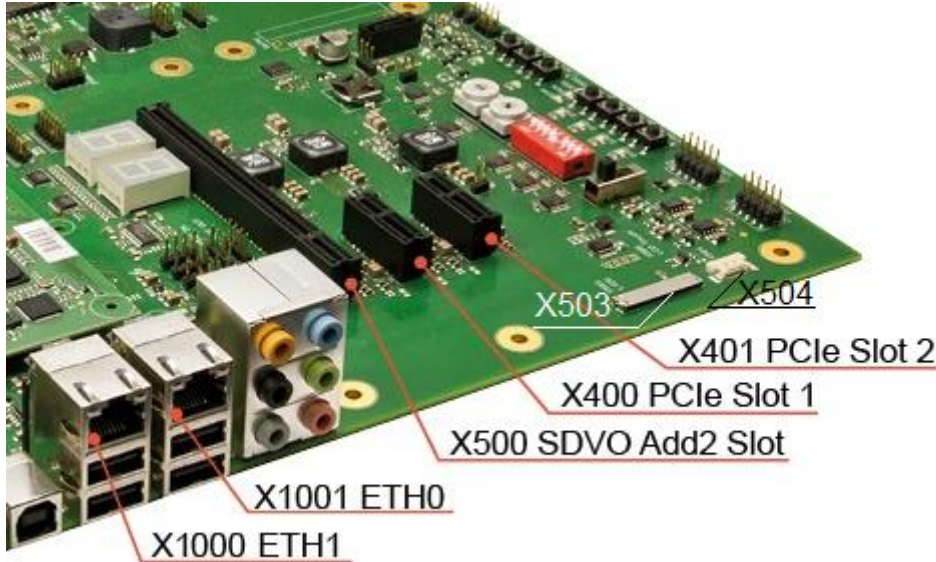
Figure 26: Connections for Keyboard, Mouse and Display to the Development Board
