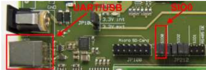
Figure 14: Jumper configuration to enable SIO0 (USB/UART)
