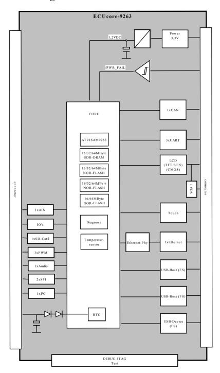
Figure 2: Block Diagram ECUcore-9263
