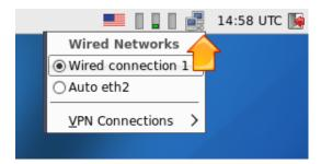
Figure 45: Changing the network configuration in the "Network Manager"
