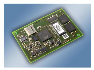
Figure 1:Top view of the ECUcore-9263
