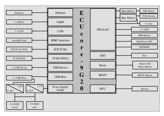
Figure 2: Block Diagram Development Board ECUcore-9G20
