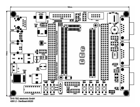
Figure 3: Positions of components
