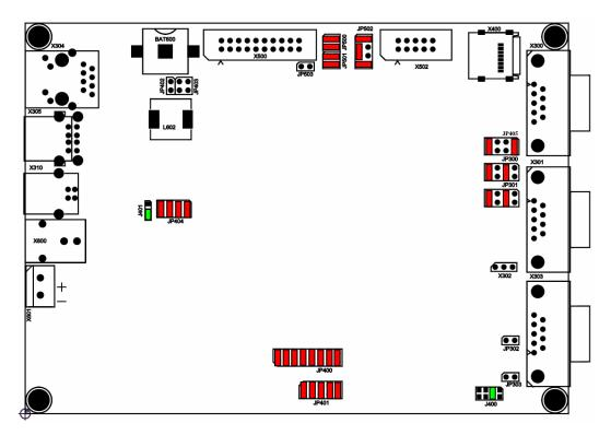
Figure 4: Default Jumper configuration
