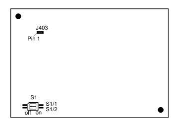
Figure 4: Jumper positions PCB 4258.0 (PLD)
