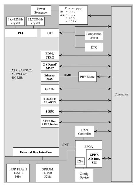
Figure 2: Block Diagram ECUcore-9G20
