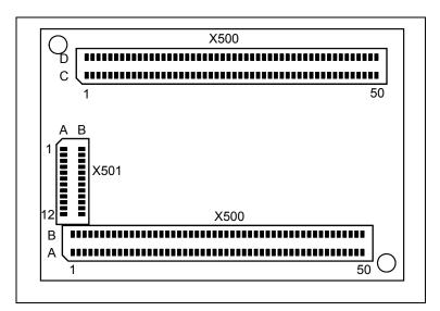
Figure 5: Pinout of the PLCcore-9G20 - top view
