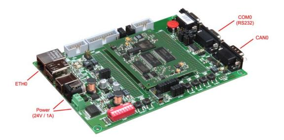
Figure 3: Positioning of most important connections on the Development Board for the PLCcore-9G20
