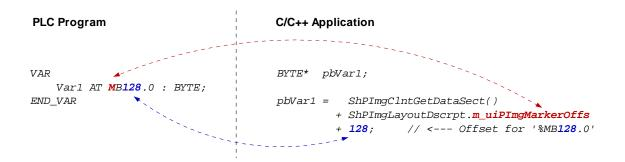
As described above, **ReadSectorTable** and **WriteSectorTable** manage the copy process to exchange variable contents between the PLC and the C/C++ program. Following the example illustrated, the Client (C/C++ application) must enter an appropriate value into the *WriteSectorTable* to transfer the value of a variable from the C/C++ application to the PLC program (*WriteSectorTable*, because the Client "writes" the variable to the Server):
