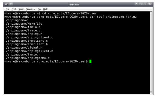
Figure 27: Unzipping the archive files shpimgdemo.tar.gz in the Linux development system
