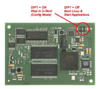
Figure 7: Positioning and meaning of DIP-Switch 1 on the PLCcore-9G20
