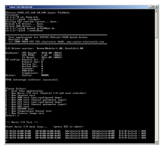
Figure 32: Testing the hardware connections using "iodrvdemo"
