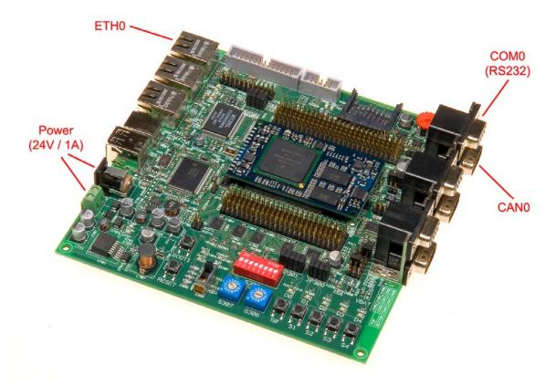
Figure 3: Positioning of most important connections on the Development Board for the ECUcore-5484
