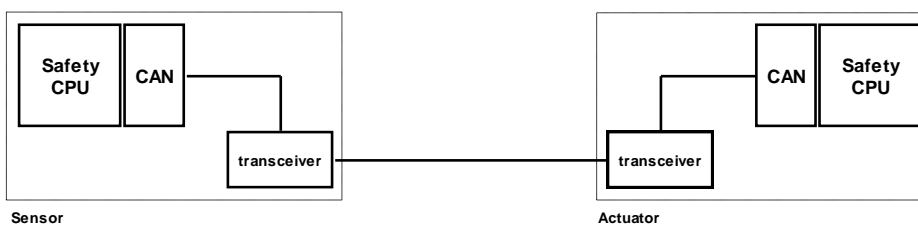
Figure 5: single-channel hardware with Safety-CPU
