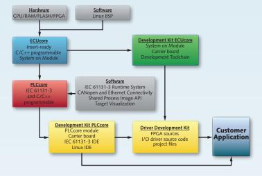
SYS TEC electronic to provide an abstract and target independent application interface to integrate user-written C/C++ application or I/O driver code. This allows for creating customized application-specific firmware versions without the need for buying an own OpenPCS development license. The Shared Process Image technology is supported by all PLCcore modules since 2007.
