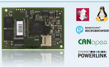
The PLCcore-9263 combines a performance-optimized and industry-proven hardware platform with the IEC 61131-3 programming environment OpenPCS by infoteam Software. The pre-installed runtime system includes CANopen and Ethernet connectivity. Open interfaces allow for extending the run-time system with own functionalities. This makes the PLCcore a most flexible controller platform.
